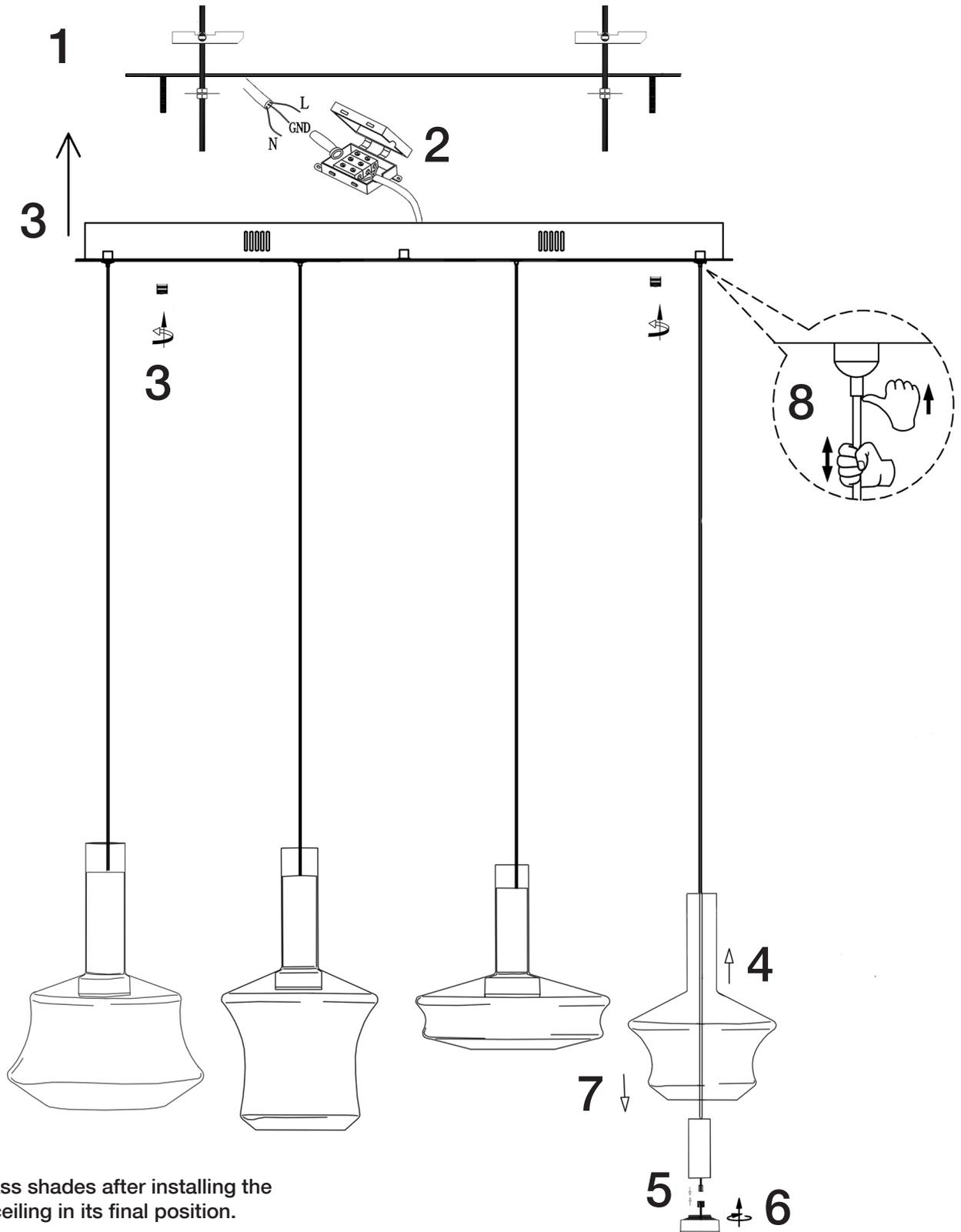
Place the glass shades after installing the lamp to the ceiling in its final position.
